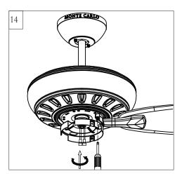
Install the blade assembly to motor using the preinstalled screws. Tighten screws securely. Repeat this process for remaining blade assemblies.
