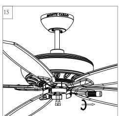
Remove set screws from top cover of switch housing. Keep screws.
