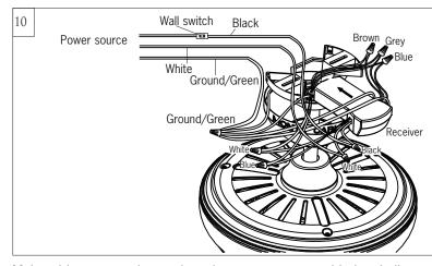
Make wiring connections using wire connectors provided as indicated above.
