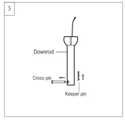
Remove preassembled cross pin and keeper pin from downrod.
