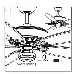
Install witch housing, aligning the holes on switch housing with screw holes on top cover. Reinstall the set screws removed in installation step 15.
