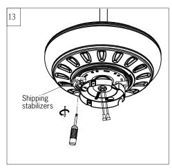
Remove shipping stabilizers from motor assembly.
